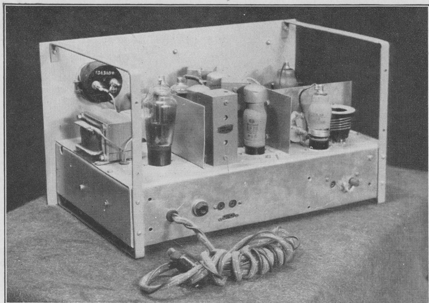
Rear view of the receiver. Note the screening of the various stages.
